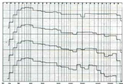
Fig. B: frequency response at 0°, 15°, 30°, 45° (external)
